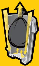
BUILT IN VENTING CHANNELS
