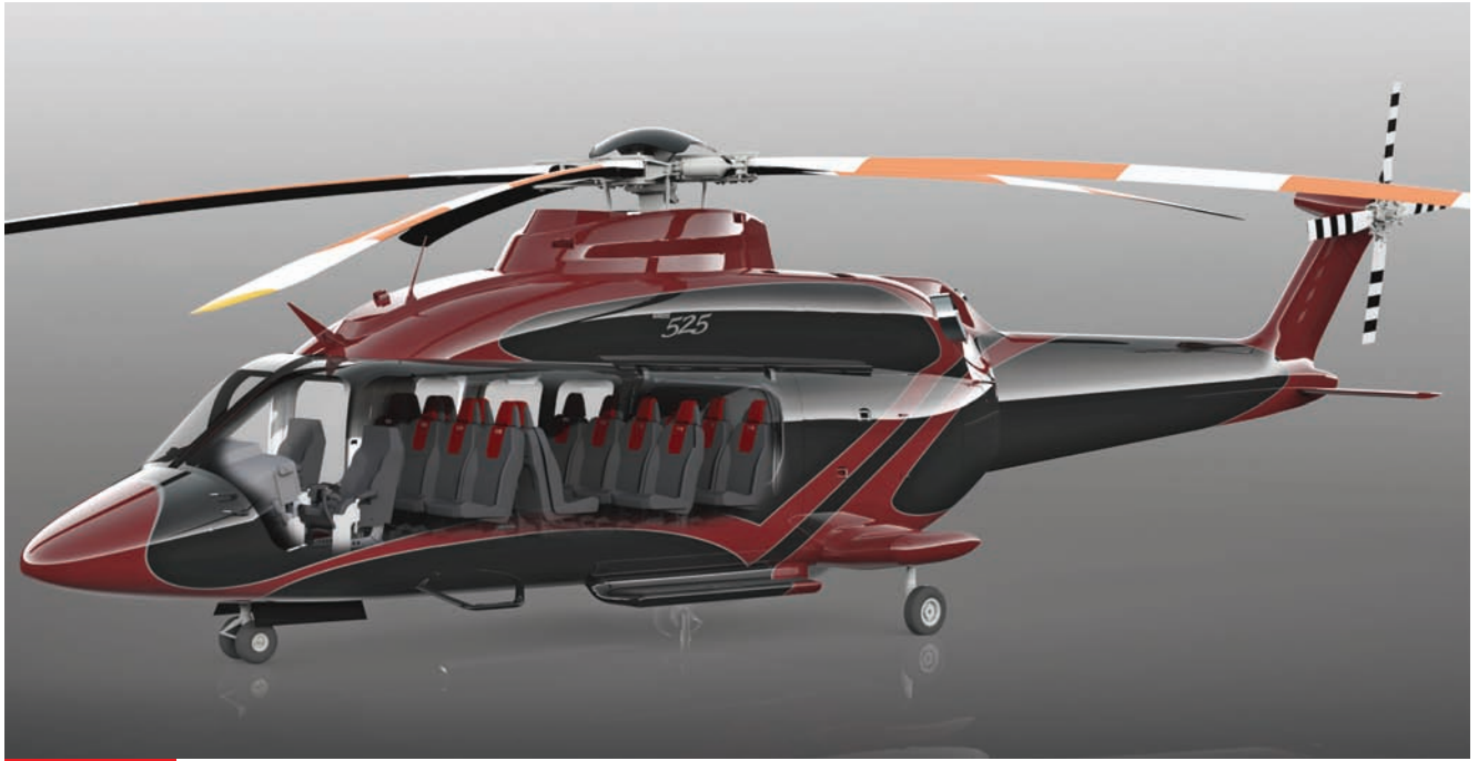
ARTIST RENDERING cutaway view showing the Bell 525 Relentless interior in a corporate seating configuration. BELL HELICOPTER
