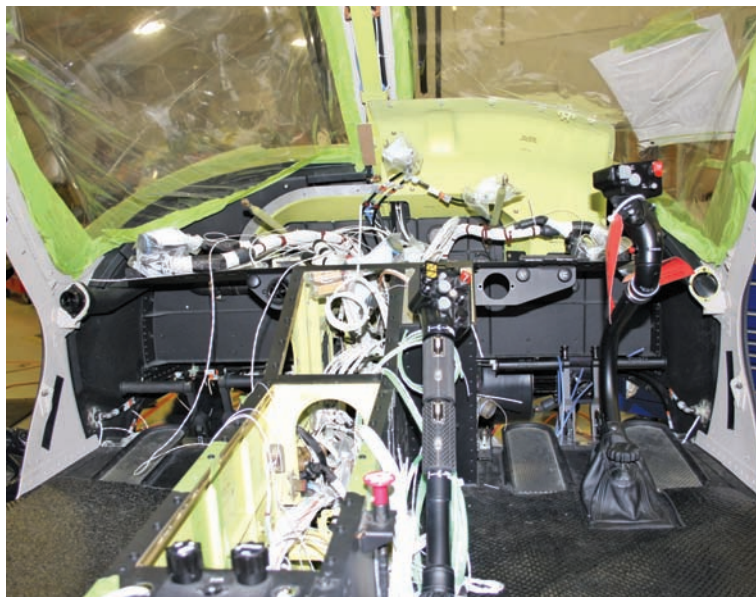
BELL HELICOPTER'S Piney Flats facility readies this aircraft for new avionics. BELL HELICOPTER
