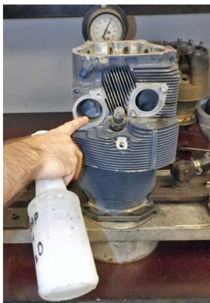
▲ THIS IS a Lycoming cylinder undergoing a leakdown test. Continental's facility rebuilds Lycoming engines. CONTINENTAL MOTORS
