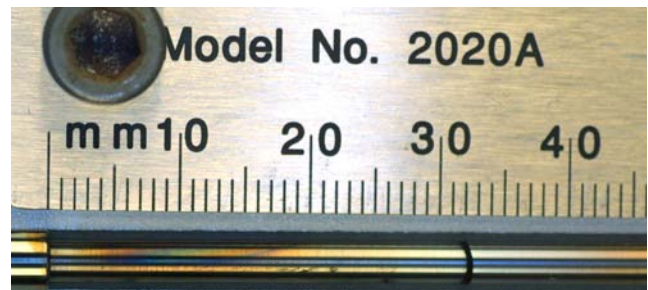
Figure 3 HPC oil in top figure, SPC shown below HLPS data contrasting coking performance for HPC and SPC oils.
