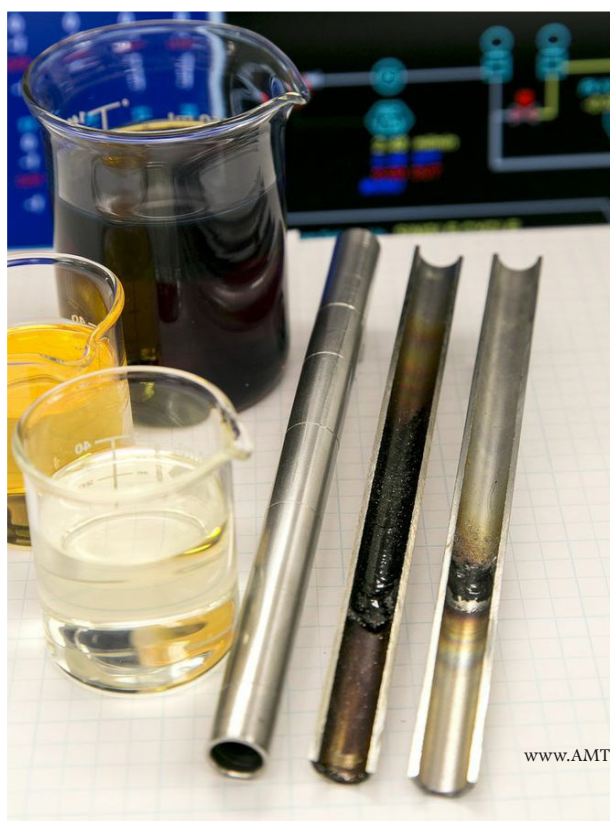
Above: Technologists review operational profile for the "Coker Mister™" Left: Example of tube deposits from a Vapor Phase Coking Test
