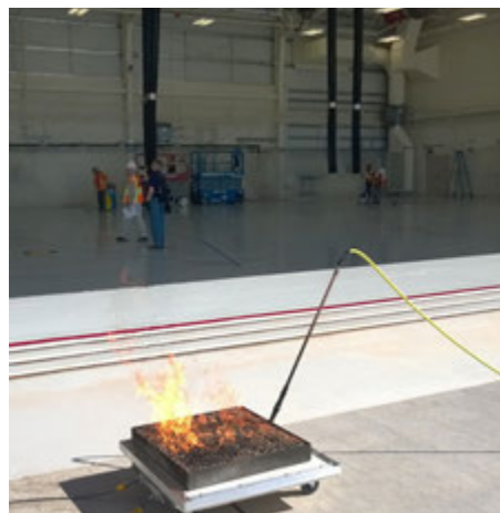
LEFT IMAGE shows the soot and smoke generated by traditional pan fire testing versus an improved proof-testing methodology using a patent-pending Jet Fuel Flame Simulator. PHOTOS COURTESY OF DET-TRONICS INC.
