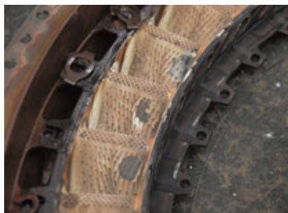
HOT-SECTION VANE as removed from the engine.
