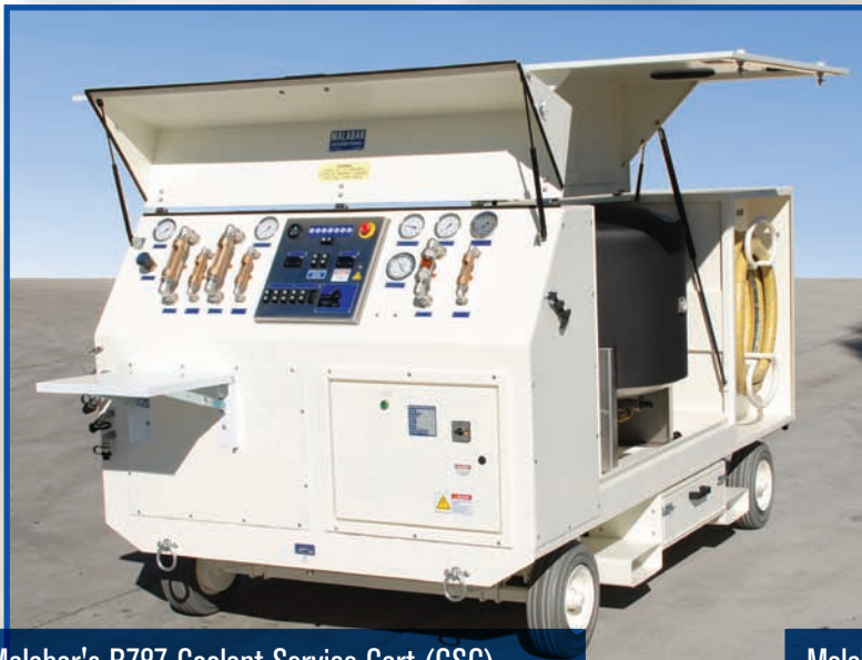
Malabar's B787 Coolant Service Cart (CSC) performs rapid aircraft coolant drain, fill, clean and de-aerate operations.
