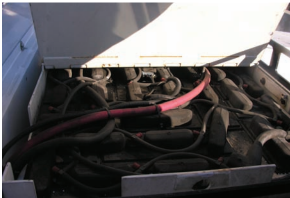
Above: an electric tug transports baggage at CLT. Left: the electric units feature a 625-amp lead-acid battery with a single-point watering system.
