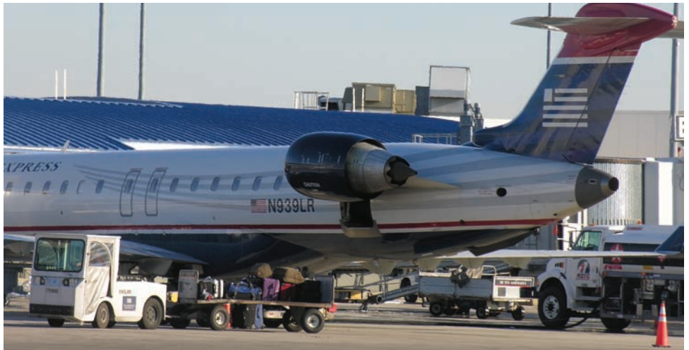
Above: an electric tug transports baggage at CLT. Left: the electric units feature a 625-amp lead-acid battery with a single-point watering system.
