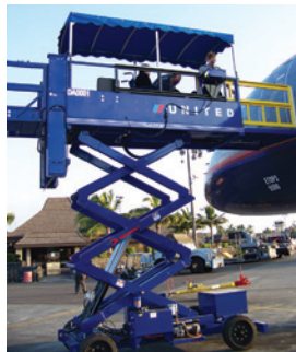
Disabled Passenger Lift
