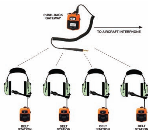
Typical wireless headset ground support communication system configuration for up to four users per gateway
