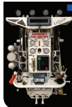
Clyde Machines Inc. displayed its new Maintenance Stand that features non-slip, self-cleaning steps and platform floor with a 500-pound capacity.
