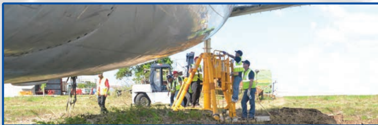
One of the Malabar rapid deployment jacks assembled and in use at a training exercise.
