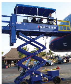
Disabled Passenger Lift
