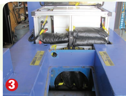
1. The Corvus lithium battery pack, with a specially designed container for the tractors. 2. A tractor integrated with the battery pack. 3. The Corvus battery integrated into a tractor with additional ballast weight for the six-month test.
