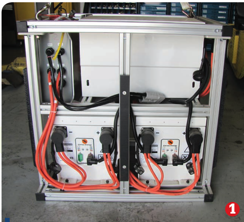
1. The Corvus lithium battery pack, with a specially designed container for the tractors. 2. A tractor integrated with the battery pack. 3. The Corvus battery integrated into a tractor with additional ballast weight for the six-month test.
