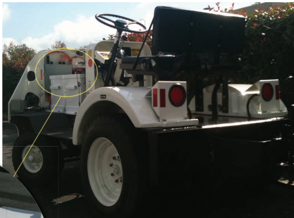
Corvus Energy plans to use this tug to test GSE powered with lithium-ion batteries. The tug uses two 48-volt, 150 amps/hour battery modules. Photo courtesy of Corvus Energy.
