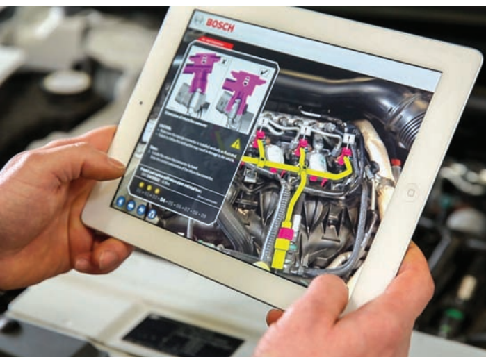
▲ Augmented reality apps, like Bosch’s iPad app seen here, make engine repair and documentation accessible anywhere. Bosch
