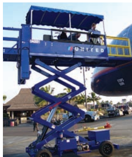
Disabled Passenger Lift
