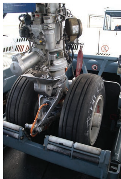
Two major components of the Taxibot make it different from other towbarless tractors: An interface mechanism clamps on the nose landing gear, which is in turn mounted on a “rotating turret.”
