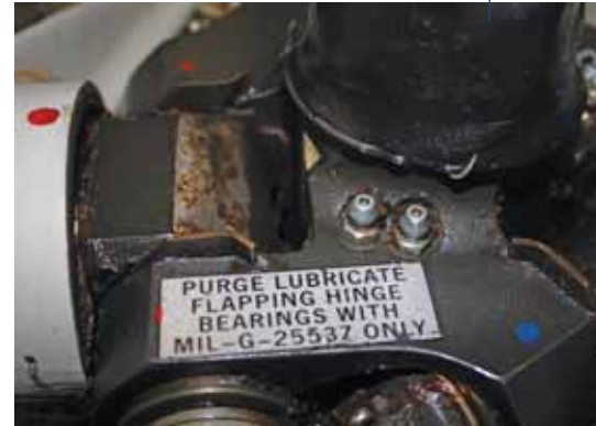
Placard showing the importance of purge lubrication on the 300CB.
