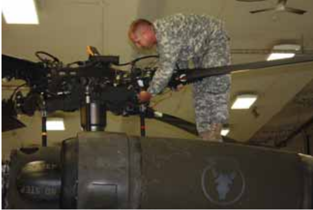
Technician Rick Gendreau accomplishing blade deice troubleshooting on the main rotor of a Black Hawk. Photo by Ronald Donner.
