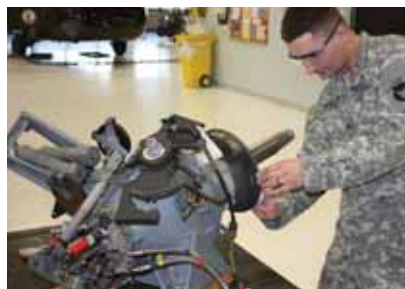
Technician Mike Ricke reassembling the tail rotor gearbox during a Phase 2 inspection. Photo by Ronald Donner.
