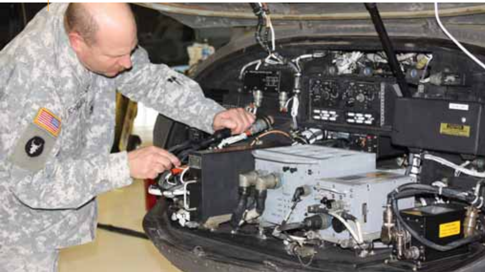
Technician Joe Schnellman working in the forward located avionics compartment of a Black Hawk. Photo by Ronald Donner.
