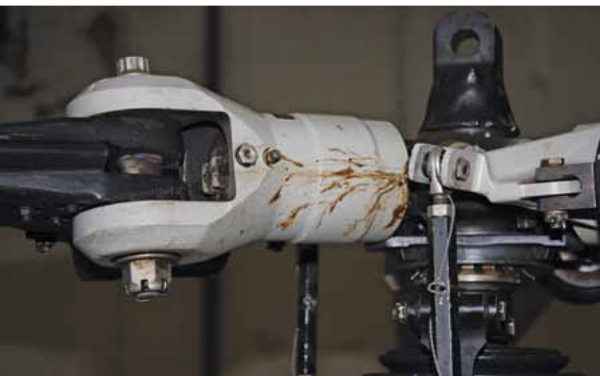
Rotating parts of helicopters generally sling grease requiring regular cleanup and re-greasing.
