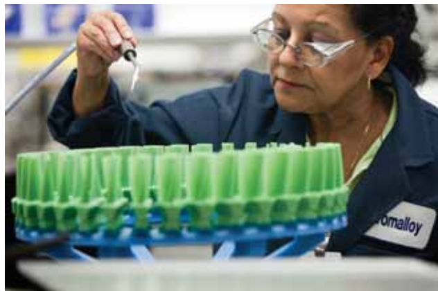
Wax patterns for turbine engine blade casting. Photo courtesy of Chromalloy.
