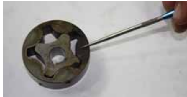
Corroded transmission oil pump rotor a common shop rejection during overhaul. Photo provided by Ronald Donner.
