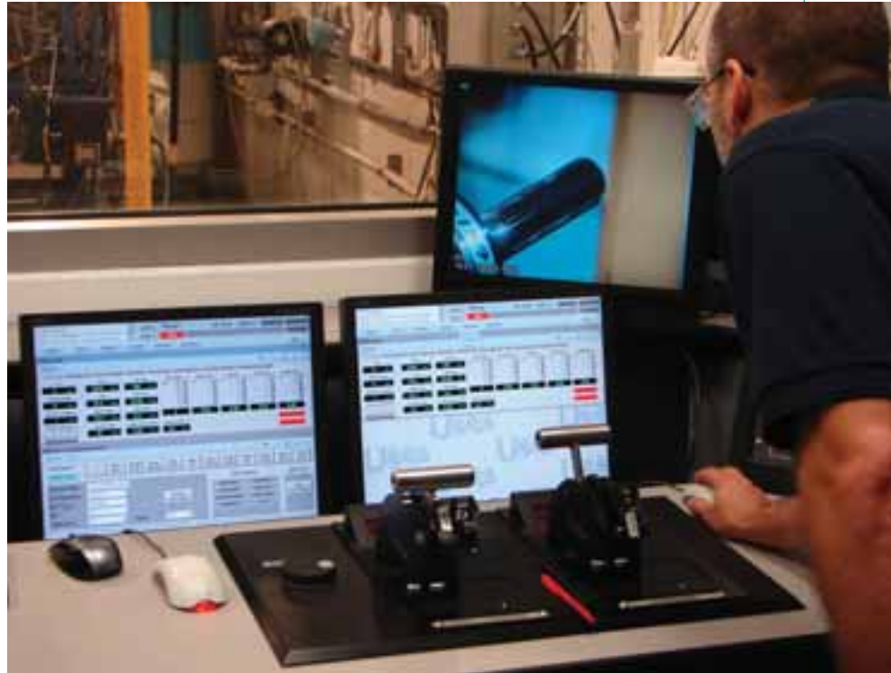
The test cell control panel in the Indianapolis Rolls-Royce facility. Photo courtesy of Tim Kern.
