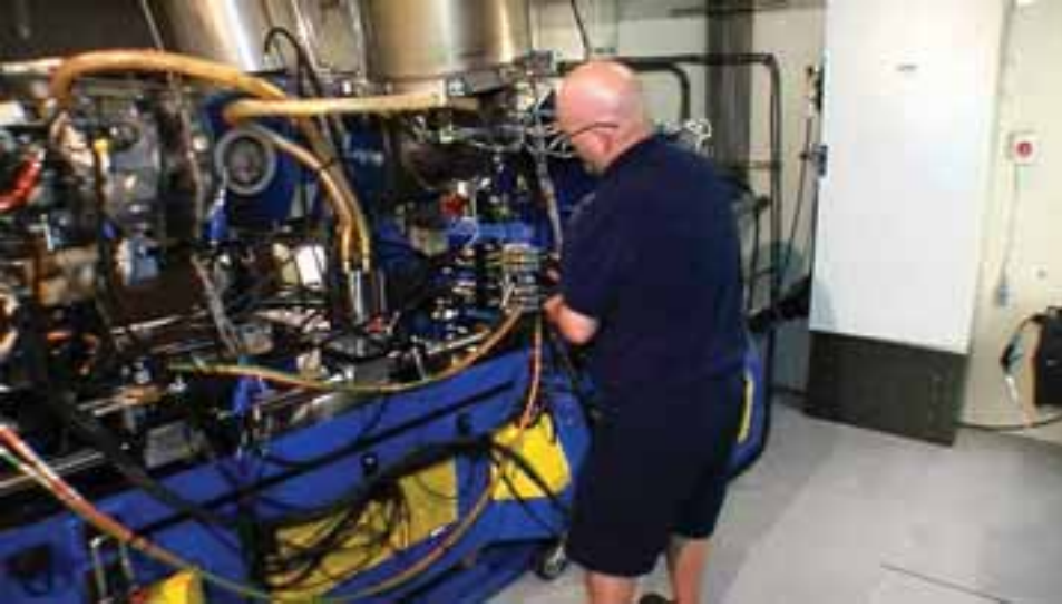
Operator preparing an overhauled engine for test in the new Timken test cell. Photo provided by Timken Aftermarket Solutions.
