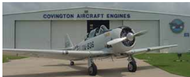
AT6 World War II trainer powered by a Pratt & Whitney radial engine. Covington Aircraft's Radial Engine Division overhauls R-985 and R-1340 engines. Photo courtesy of Covington Aircraft.
