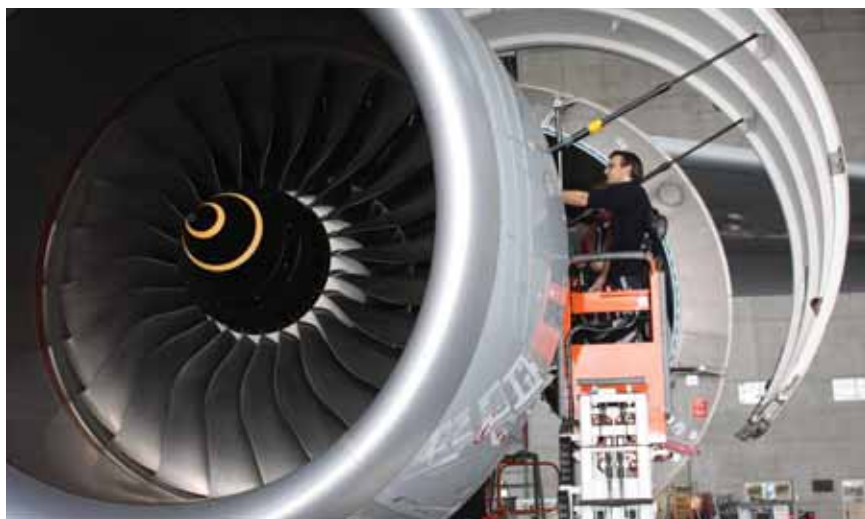
Lufthansa Technik technicians troubleshoot a No. 1 engine speed sensor fault on the A380 in Frankfurt, Germany.
