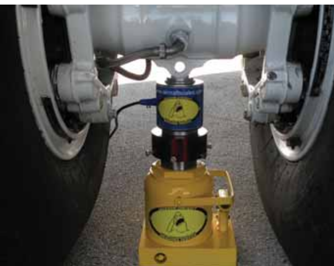
A top of jack cell-based scale used on a B727 main landing gear. Photos courtesy of Larry Jackson.
