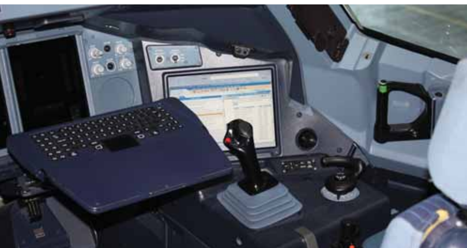
Maintenance data can be accessed in the A380 cockpit via the onboard information system.
