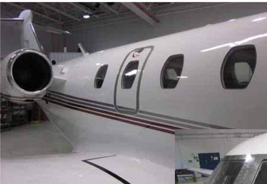
Passenger cabin windows and cockpit windshields on a Cessna Citation III aircraft. Photos courtesy of Signature TECHNICAir - STP.
