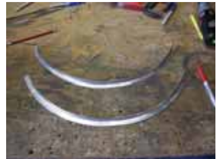
Curved sections fabricated by shrinking and stretching.
