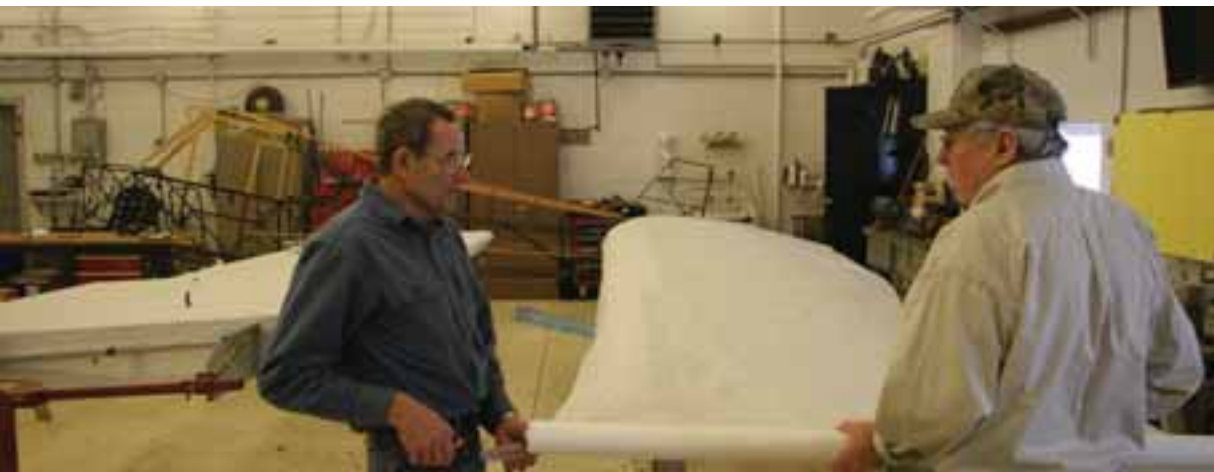
Hank Geissler and Pat Watson discussing fabric layout for J-3 wing.
