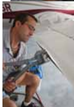
Rob Behrend using his shrinker-stretcher tool.
