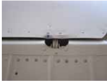
Typical example of bent thin aluminum skin.
