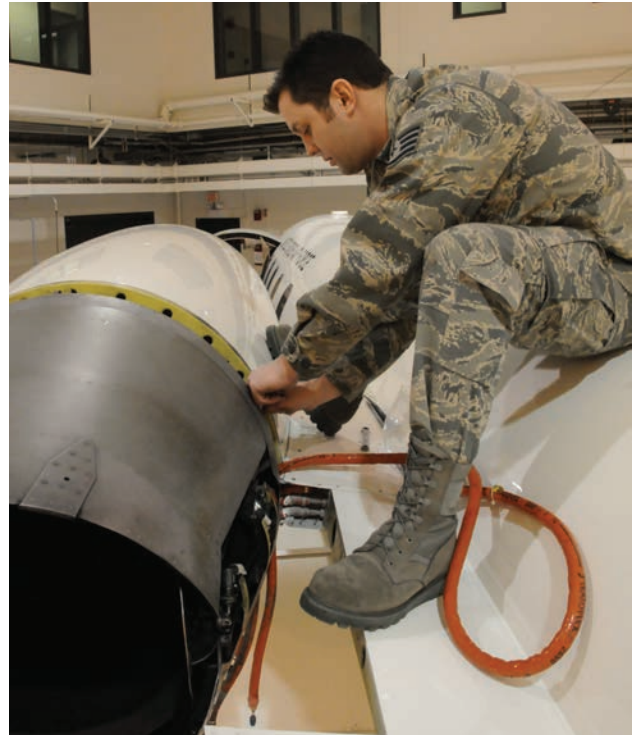
Staff Sergeant Eric Hoff installs thrust reverser flange bolts. The fire sleeve is for a wiring harness to be installed later.
