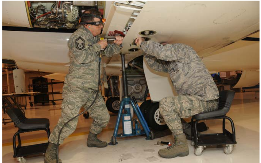
Senior Master Sergeant Kevin Odegaard and Master Sergeant Jeff Lien buck rivets on a flap sector bracket replacement.
