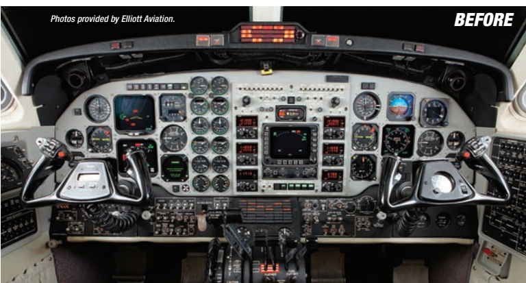
King Air 350 instrument panel before the retrofit.
