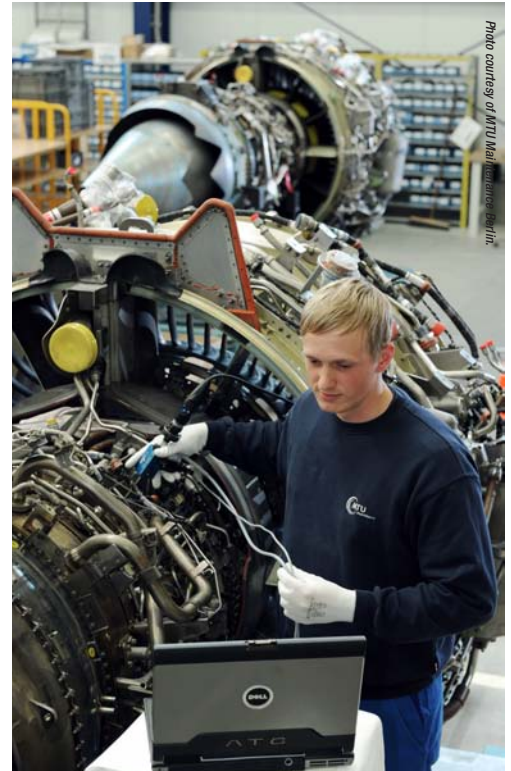
The CF34 inner workings being inspected in the MTU Maintenance Berlin-Brandenburg facility in Germany.
