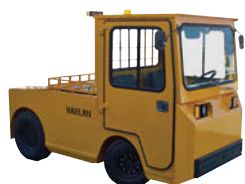
Charger Electric Baggage-Cargo Tractor Model HLE Available with lead-acid or lithium battery
