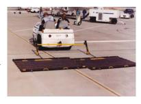
square meters (3 million square feet) per hour, at speeds from 6 kph (4 mph) to 40 kph (25 mph). Aerosweep Pty. Ltd. has released the latest improvement to the FOD BOSS speed sweeping system: the Phase Three Retention Blade (P3R). The latest technology provides even greater FOD collecting and retaining capability with new built in ribs.
