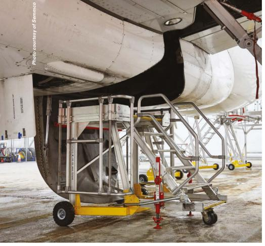
maintenance work are similar to those found in construction. However, the nonlinear shape of aircraft and the intricate maintenance tasks that must be carried out without causing any damage to the surface or structure of the aircraft can create difficult working environments that could pose additional risks. Much of this maintenance work will include working at height, so it is imperative that the maintenance engineers can work, know-
