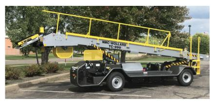
feature colored and marked wiring, automotive electrical connectors, circuit breakers and fuses, CANBUS communication between engine, transmission, smart switches and Belt Control Unit, LED lighting throughout the vehicle – in essence, the TC–999 is similar to working on a new car. Hydraulic components have been upgraded, a reservoir that utilizes a filter, fully integrated within the reservoir tank, eliminating external valves and hoses previously used," describes McDermott.
