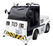
JET-16 and will integrate all remote control, communication and safety detection tools developed by EasyMile as part of their driverless technology.
