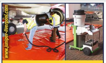
In addition to the mat with inflatable sides on our Kyoto waste water collection trailer, we now have a stand-alone mat (SM 895-02) with insertable foam sidewalls and a self-powered vacuum unit (SM 939).
