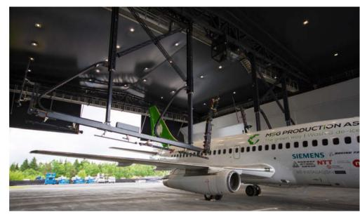
The environmental benefits of the MSG are multifold. Being inside a hangar allows for the easy capture and containment of ADF and an on-site recycling system makes for quick processing of the fluid, which can then be resold. The automatic nature of the MSG also ensures only as much deicing fluid as needed is sprayed.
