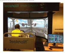
immersive training experience. TecknoSIM simulates both towbar and towbarless pushback equipment.
