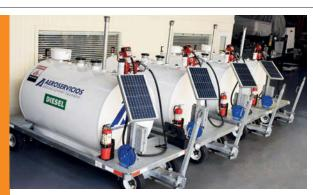
Specially designed by end users, mechanics and engineered by our team of GSE experts. 550 Gal Diesel or Gasoline, double wall UL Tank, solar powered pump 15 GMP. in f 🛛 🔽 🖸
