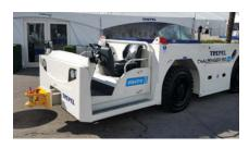
front axle suspension provides driving comfort for the operator. Options include open drivers stand with side safety bars and solid tires.
