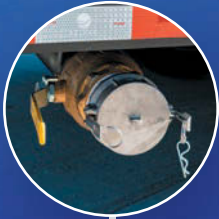
WASTE DRAIN 4" BALL VALVE
