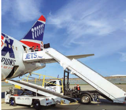
Construction of Stinar's SPS-3518 includes a steel frame with aluminum panels, diamond plate steps and platform, and stainless steel handrails.
