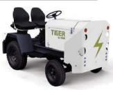
maintenance. These tractors maintain uncompromised range, towing and hauling and offer familiar operator user controls for seamless GSE adoption. Tiger Li-ion tow tractors are built on industry-proven steel chassis, with up to 60,000 pounds towing capacity, hitch options, color choices and durability features.
