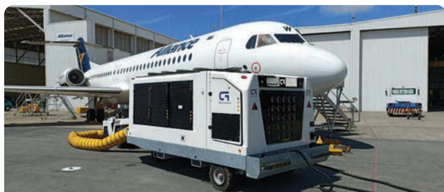
The modular construction of the GF15 Combo Unit optimizes maintenance access.
