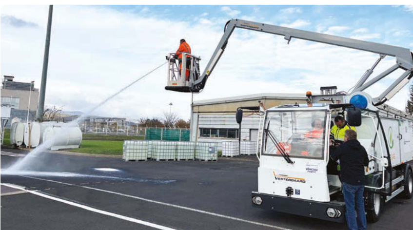
The Elephant e-Mini MY Lite is a simplified, off-the-shelf version of the traditional Elephant MY introduced especially for servicing smaller to medium-sized aircraft.
